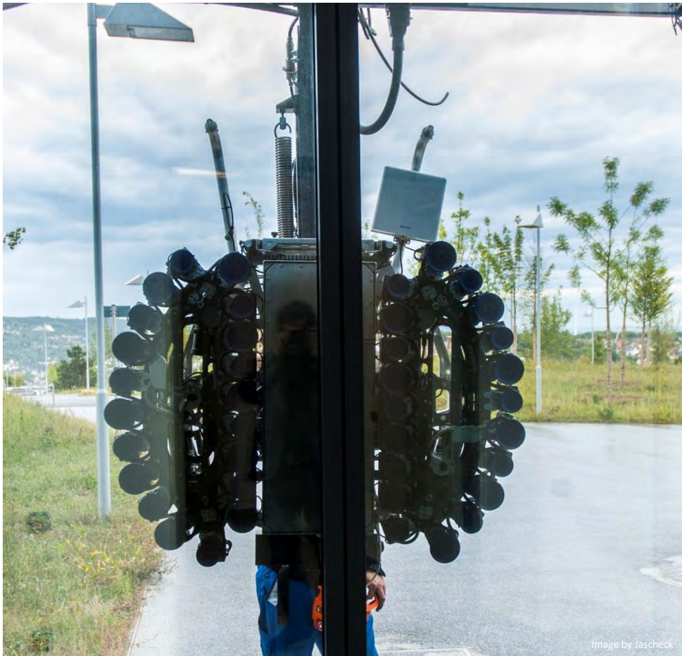
Automated robot cleaning, view from inside
