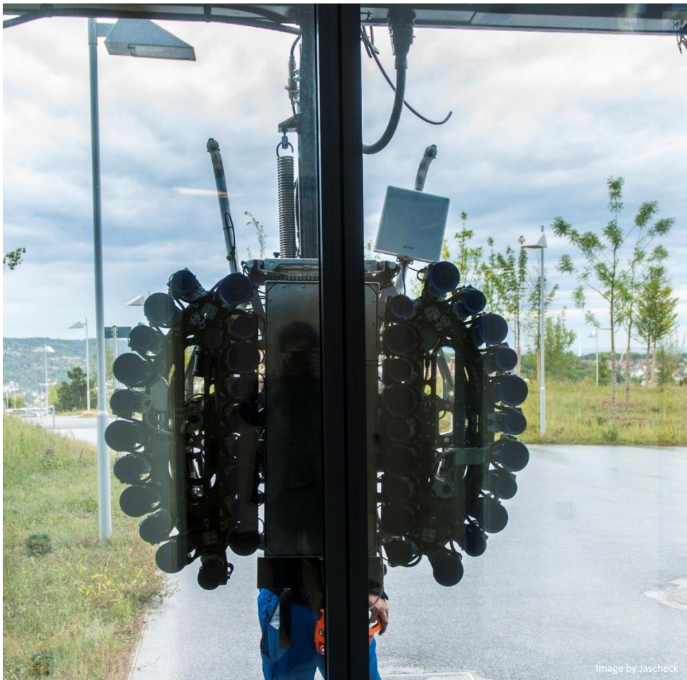
Automated robot cleaning, view from inside
