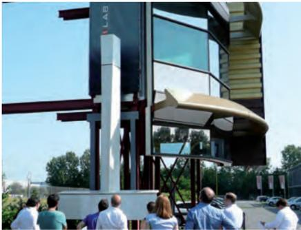
Thanks to technical, manufacturing and planning know-how and support from local partners the Facade-Lab is able to produce prototypes and Mock-Ups to realistically evaluate newly developed building skins in early stages of construction and research projects.
